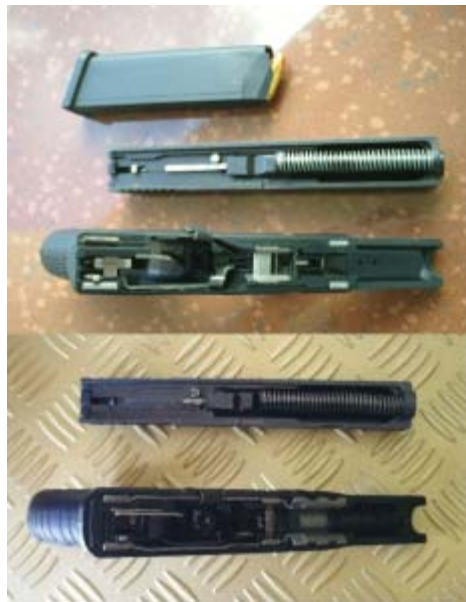
Inside out: The internals of this early model Glock [top] is strikingly similar to that of this current model Tara [above]. But the Tara appears to have more steel on the lower assembly. (Photos by IGG)
